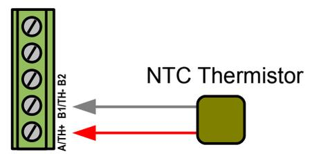
\* When the wire length is long, shielded cable is recommended.
