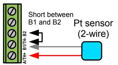
\* When the wire length is long, shielded cable is recommended.
